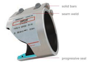
Each coupling (whether Axilock or Axiflex) consists of a casing, a gasket and a lockpart. The purpose of the casing is to house the gasket and to press it onto the pipe surface when the lockpart is closed. The lockpart is designed to pull the two ends of the casing together circumferentially around the pipe. In order to achieve this, the coupling is labeled clearly with a torque figure which ensures that the gasket is compressed sufficiently against the pipe surface.
