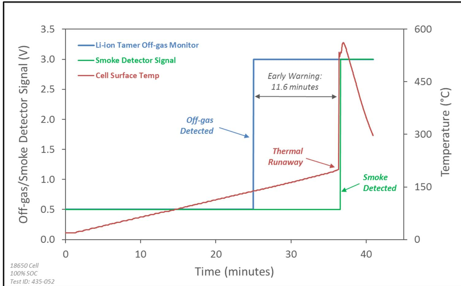
Off-gas can be detected prior to thermal runaway
