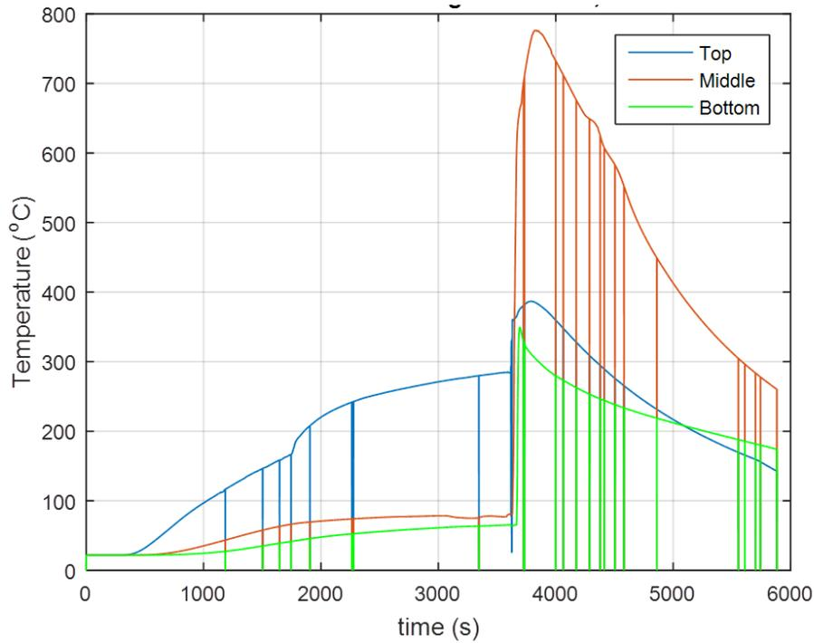
Figure 14 Results from stacked cell test, 75 Ah NCM Li-ion pouch cells.
