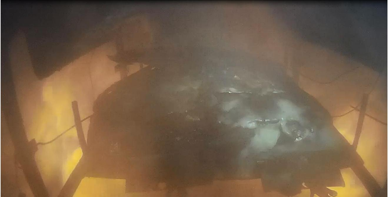
**Figure 10** Time 80: Flashover as oxygen is introduced
