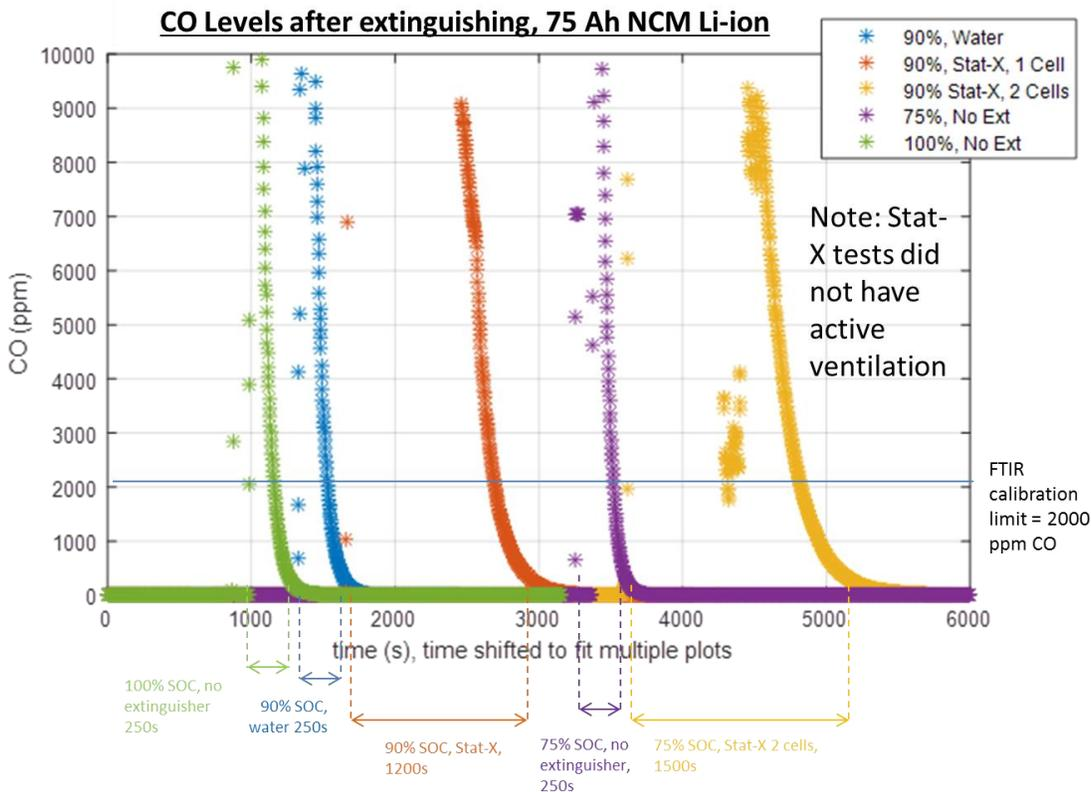
**Figure 16** CO levels after extinguishing for several tests on the 75 Ah NCM Li-ion cell.
