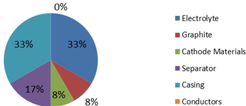
**Figure 2** Approximate composition by mass percentage for Li-ion batteries.
