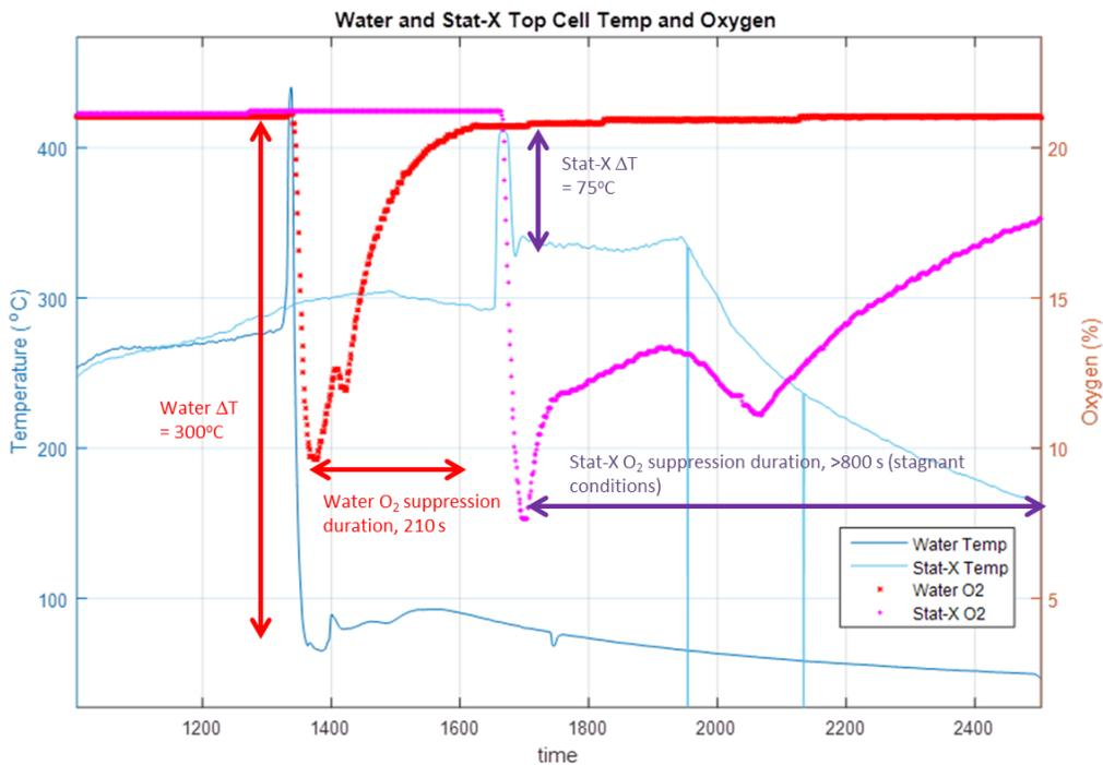
Figure 15 Water vs. Stat-X in cooling capability and oxygen suppression for the 75 Ah NCM Li-ion cell.
