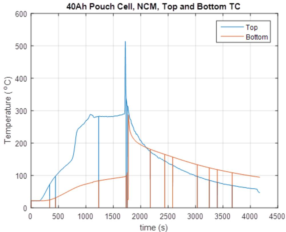
**Figure 12** Battery cell temperatures above and below the cell during Stat-X extinguishing.
