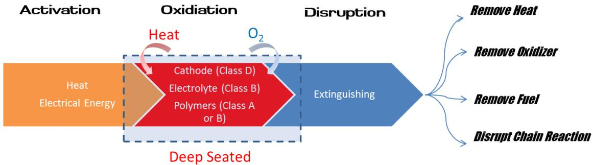
**Figure 3** Stages of a Li-ion battery fire and mechanisms for its propagation and extinguishment.
