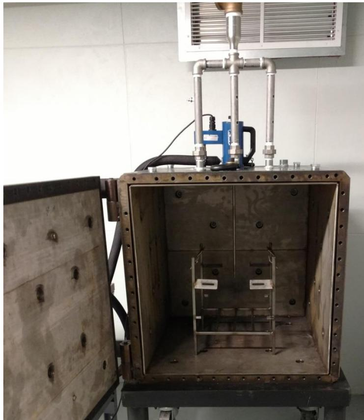
**Figure 5** DNV GL's large battery abuse chamber is designed to hold battery cells on a rack with radiant heating from above, while temperature are monitored at multiple locations and the FTIR gas monitoring probe extends from above.
