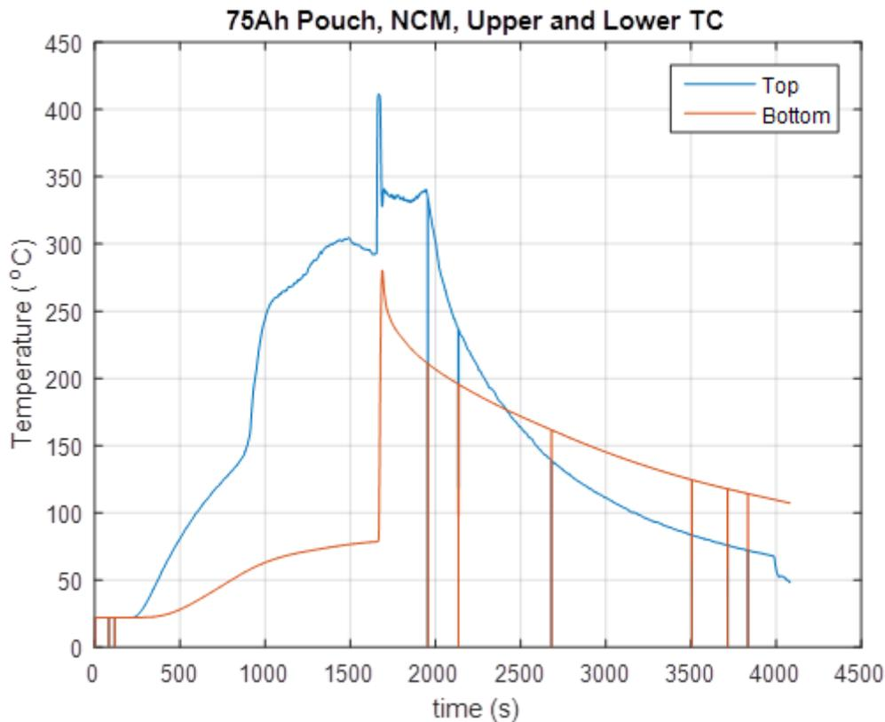
**Figure 13** Stat-X temperature performance for a single 75 Ah NCM Li-ion pouch cell.
