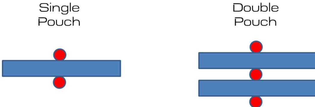
**Figure 4** Cell tests were conducted with thermocouples (red) monitoring the upper and lower surfaces of a single pouch (left), as well as scenarios simulated packed pouches in a battery module with thermocouples monitoring the upper and lower surfaces as well as the interior (right).
