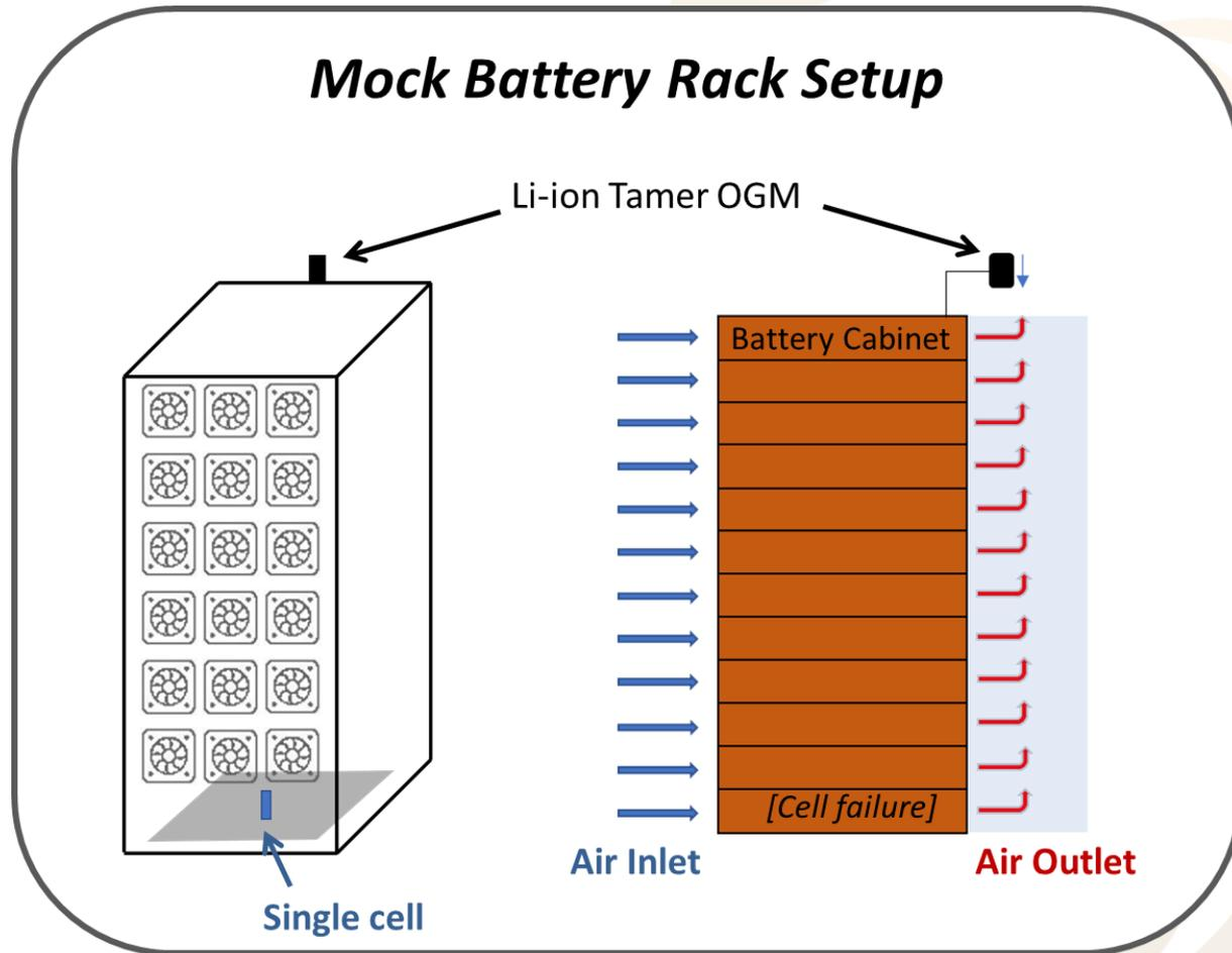
Test set up used to demonstrate single cell detection in battery rack with one Li-ion Tamer off-gas monitor
