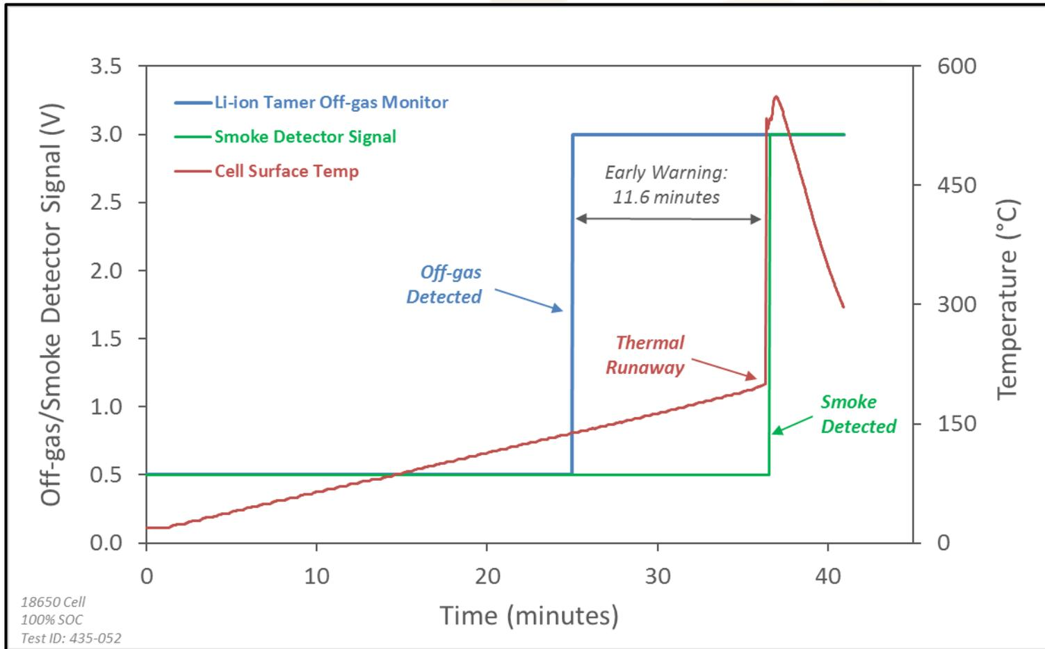
Li-ion Tamer<sup>®</sup> detects off-gas *prior* to thermal runaway
