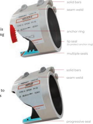
Each coupling (whether Axilock or Axiflex) consists of a casing, a gasket and a lockpart. The purpose of the casing is to house the gasket and to press it onto the pipe surface when the lockpart is closed. The lockpart is designed to pull the two ends of the casing together circumferentially around the pipe. In order to achieve this, the coupling is labeled clearly with a torque figure which ensures that the gasket is compressed sufficiently against the pipe surface.
